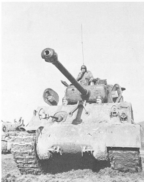
M4A3 SHERMAN TANK WITH 76-MM. GUN
