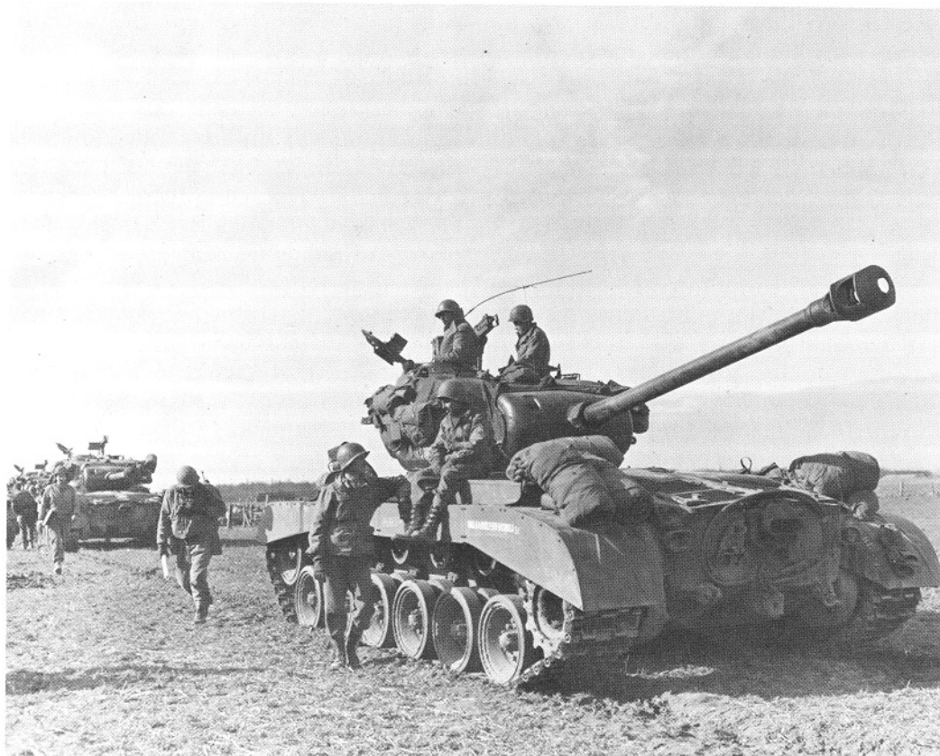
PERSHING TANK T26 WITH 90-MM. GUN
